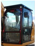
Installs easily using CAT factory mounting locations (PART# ETCG-FZT, ETCG-NGZT)
