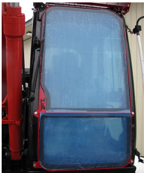
Window is pictured with blue protective film, which is removed after installation.
