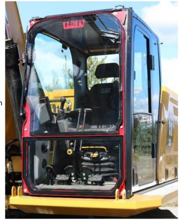
PLEASE NOTE: The windshield wiper located in the upper right- hand corner, looking out of the machine, will work with this window. Other optional wipers may not work. Due to ongoing new options offered by machine manufacturers, optional wipers, lights, visors, and cameras may not work with this window. Custom mounting or modifications may be required after the Ballistic window is installed.
