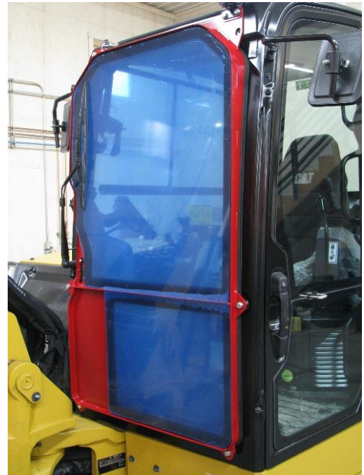
Window is pictured with blue, protective film. Film is removed after installation.
