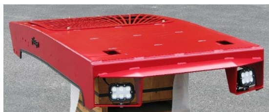
Back view of Elite Top Cab Guard. Ballistic lens covers and pigtails for lights included. Lights not included.
