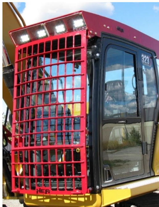
Skeleton Window Guard is shown with our Elite Top Guard and OEM window. Note! Guards are shown in red for illustration purposes only. Guards are painted black.
