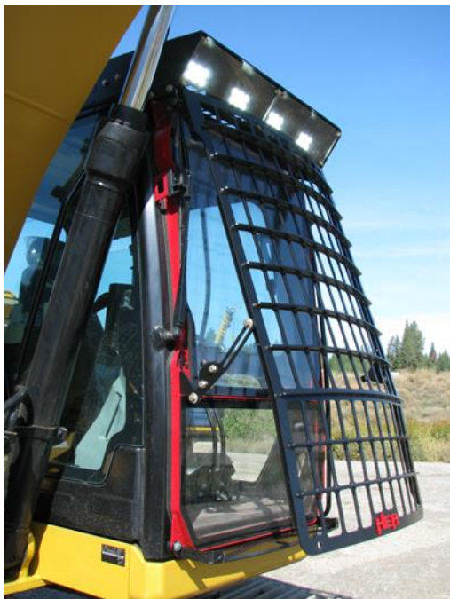
Skeleton Window Guard (hinged open) is shown with our Ballistic Defender Window and Elite Top Guard.
