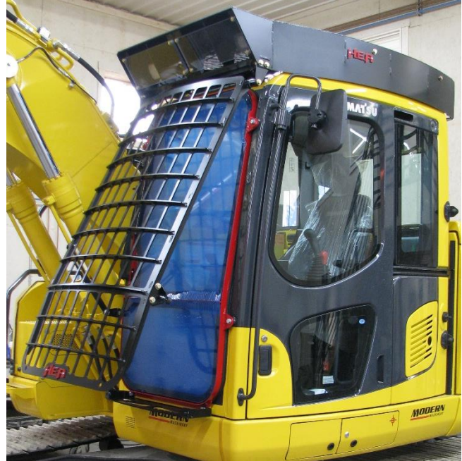
Skeleton Window Guard shown (hinged open) with our Ballistic Defender Window and Elite Top Guard. Note! Window has blue protective film on it used for shipping purposes.
