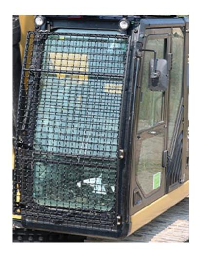
**PLEASE NOTE**: Due to ongoing new options offered by the machine manufacturer, lights, visors, wipers, and cameras options may not work with this window guard. Custom mounting or modification may be required to these options after the guard is installed.
